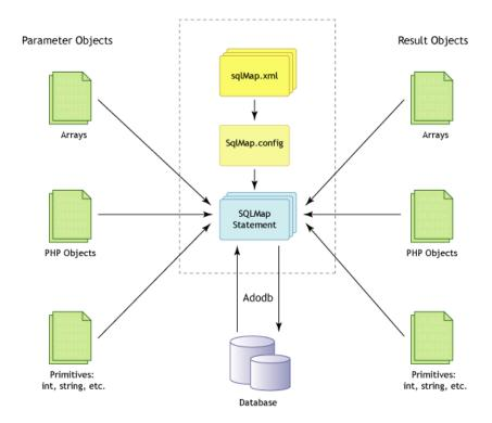
Here's a high level description of the work flow illustrated in the figure abov. Provide a parameter, either as an object or a primitive type. The parameter can be used to set runtime values in your SQL statement or stored procedure. If a runtime value is not needed, the parameter can be omitted.
